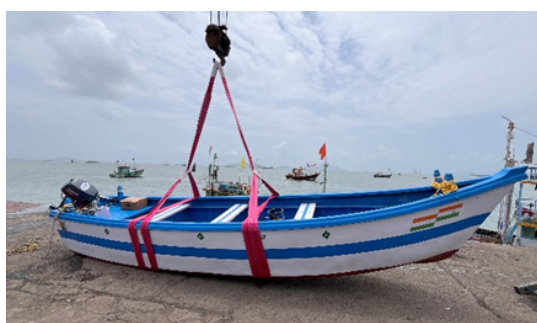
9.9 HP LPG-retrofitted boat
