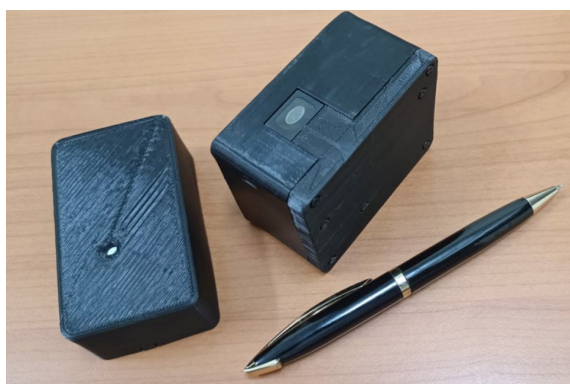
Handheld portable NIR device for on field non-destructive quality evaluation of seafood
