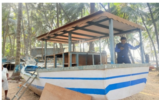
Series hybrid electric boat - 20 HP
